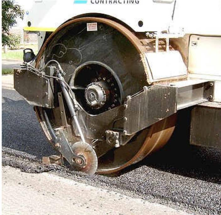
Figure 8. Cutting Wheel Fixed to Roller in the United Kingdom
